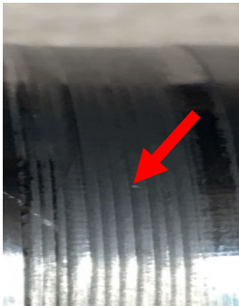
Heavy Tool Lines Unacceptable
