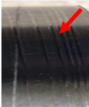
Spiral lines, not continuous (may meet surface finish) Unacceptable
