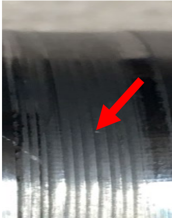
Heavy Tool Lines Unacceptable
